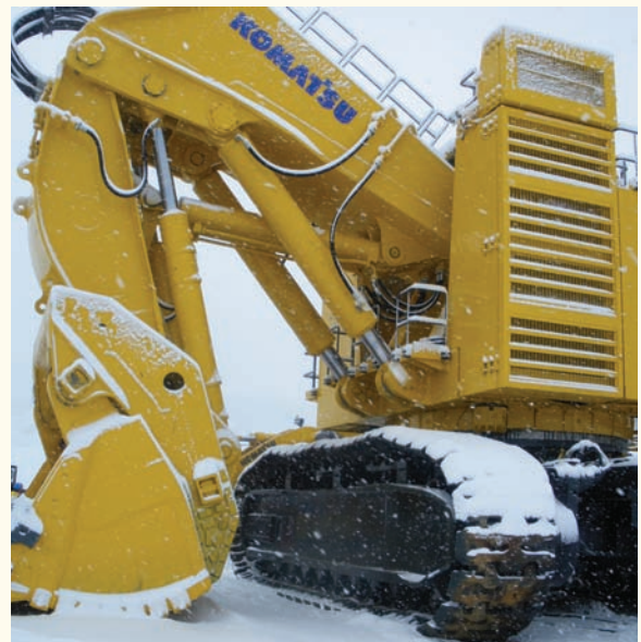
Copper Mountain took delivery of a Komatsu PC8000 mining shovel in November, part of a fleet of Komatsu equipment that will be operating at the mine.
