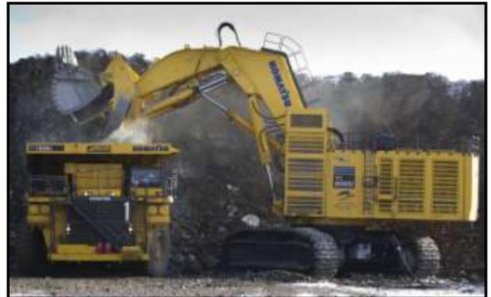
*Picture Above: PC 8000 loading 240 ton haul truck*
