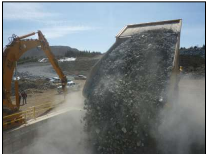
Picture Above Left and Right: 240 ton haul truck dumping first load of ore into the Company’s new primary crusher
