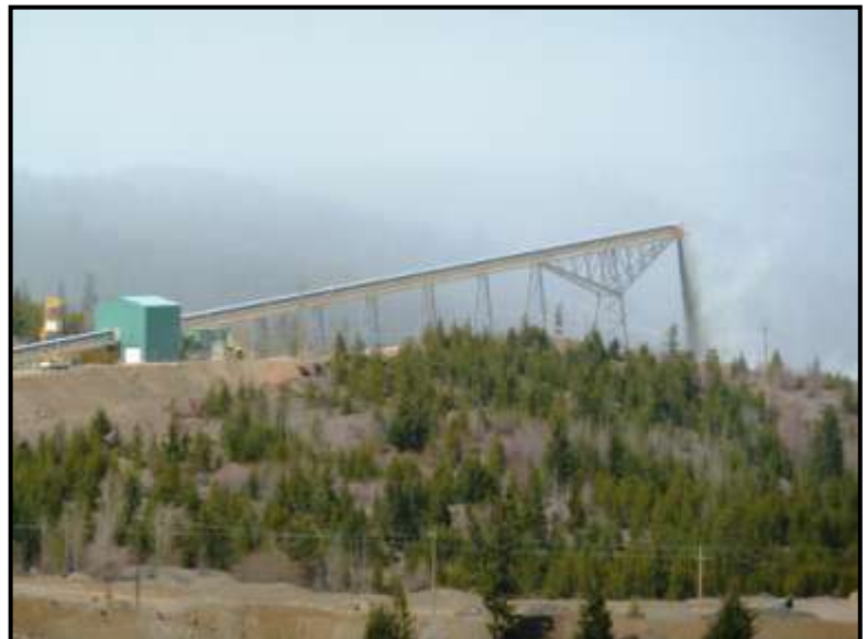
Picture Below: Overland conveyor system transporting crushed ore to the coares ore stock pile adjacent to the concentrator
