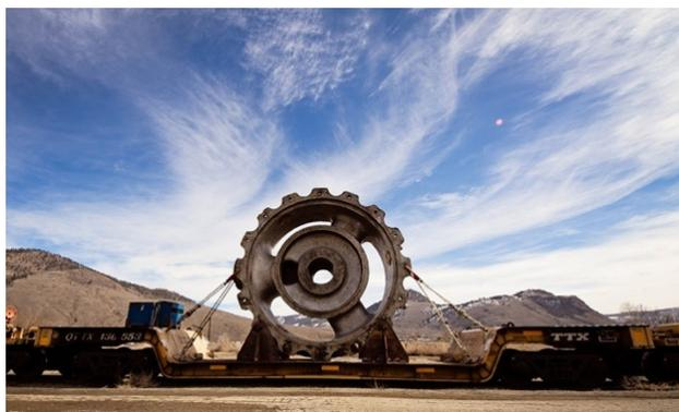
The lower bowl frame of the secondary crusher in Kamloops, B.C., is waiting to be transported to Copper Mountain.
