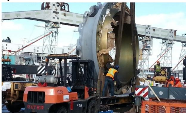
The secondary crusher's upper main frame is unloaded at the Port of Halifax for transport via rail car to Kamloops, B.C.
