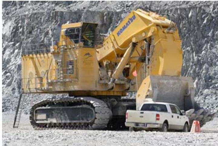
*The Copper Mountain Mine near Princeton operates two of the largest hydraulic shovels in the world - electrically powered Komatsu shovels with a 45 cubic metre capacity - large enough to swallow the pickup truck parked in front. The mine's scale - both economic and physical - is impressive, providing an economic boom to the Princeton area.*
