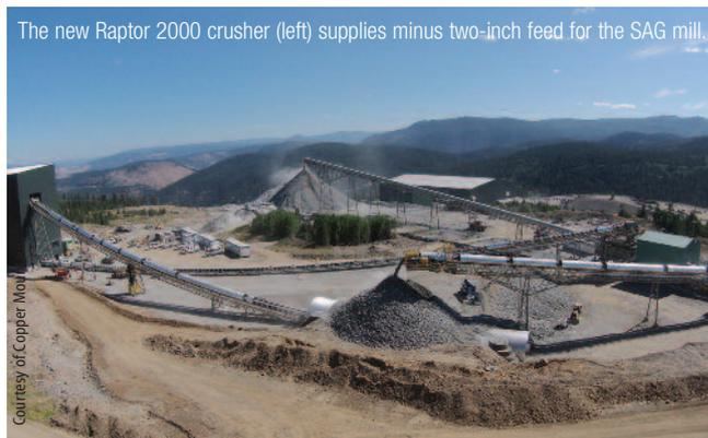
The new Raptor 2000 crusher (left) supplies minus two-inch feed for the SAG mill.
