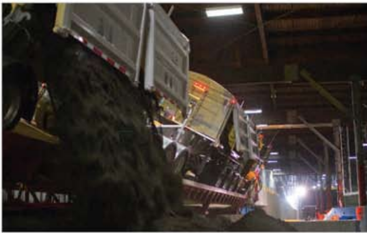
Once at the Vancouver Port, the trucks unload on a tipper. The concentrate is then shipped to Mitsubishi's smelters in Japan. Photo courtesy Copper Mountain Mining Corp.
