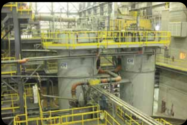
The froth flotation columns are an integral part of the mineral processing circuit at the Copper Mountain Mine.
